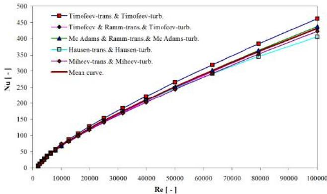
**Fig. 1.** Nusselt Number Comparison from Different Critical Equations. Transition to Turbulent and Turbulent Fully Developed Flow inside of Circular Tubes – Pr = 5
