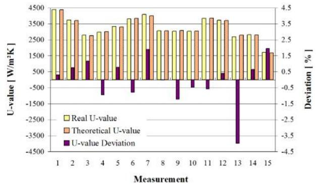
Fig. 5. Comparison Between Theoretical and Real U-values. M6-MFG Heat Exchanger – INCERC Laboratory Stand
