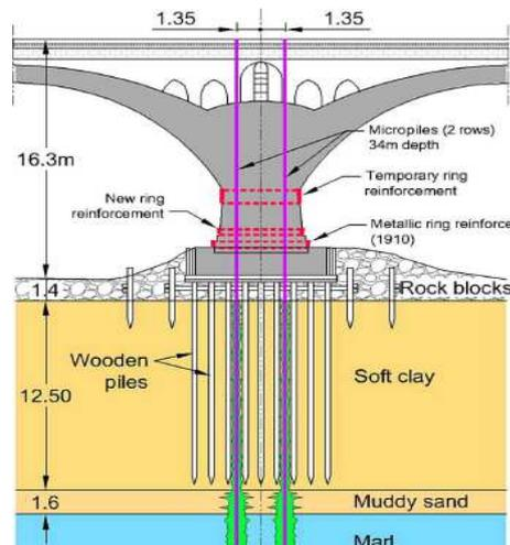
**Fig. 14.** Vertical section of Pierre Bridge in Bordeaux (Frank, 2006)
