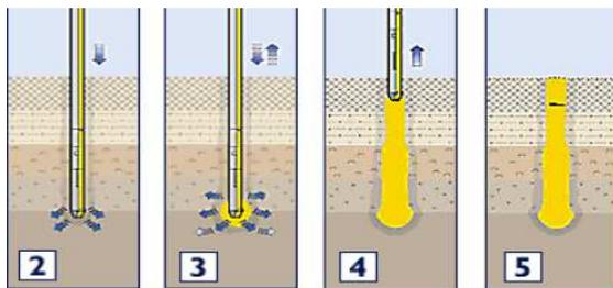
**Fig. 8.** The principle scheme of using vibro-compacted concrete columns (Briancon, 2002)
