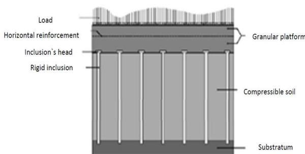
Fig. 4. The principle of soil reinforced by rigid inclusions (Chevalier, 2008)
