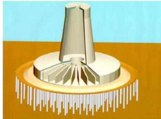
**Fig. 9.** Soil reinforcement for a pile bridge: Rion - Antirion, Greece (Auvignet, 1999)
