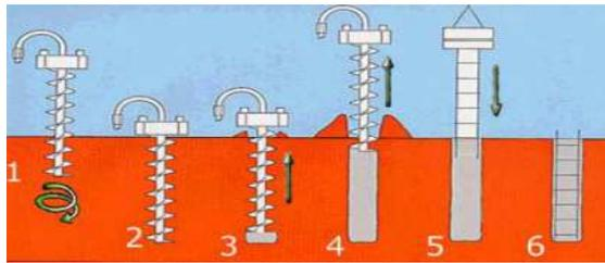
**Fig. 7.** Schematic diagram for using continuous flight auger (CFA) piles (Briancon, 2002)
