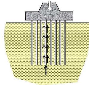
Fig. 5. Simplified scheme of a deep foundation (Hassen, 2006)
