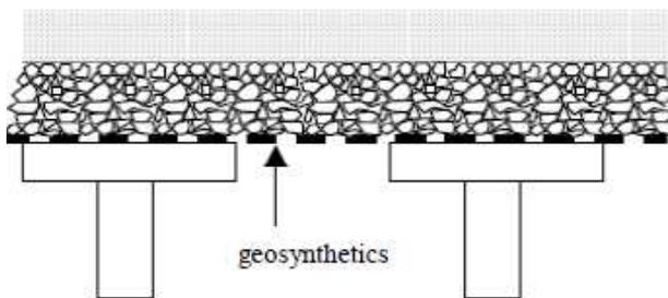
**Fig. 10.** Layout of horizontal reinforcements directly on the heads of inclusions (Briancon, 2002)
