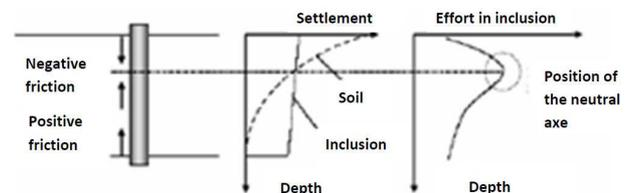
Fig. 6. Friction force along the inclusion (Berthelot et al., 2003)
