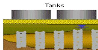
Fig. 2. Foundations for storage tanks (Briancon, 2002)
