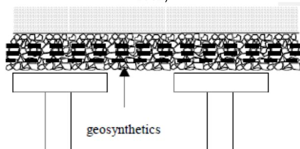
**Fig. 11.** Layout of horizontal reinforcements inside the granular platform (Briancon, 2002)
