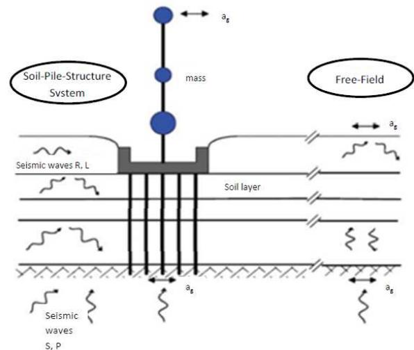
Fig. 15. Soil-structure interaction (Hatem, 2009)
