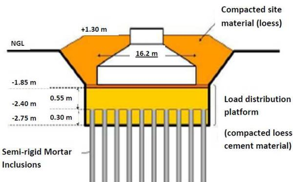
**Fig. 13.** Section for improving soft soils for foundation of wind turbines in the Dobrogea region (Menard, 2008)
