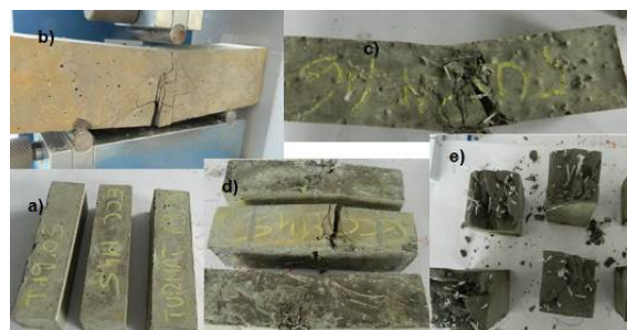
Fig. 6. Flexural test: a) specimens before tests; b) flexural loading; c) and d) rupture; e) fiber distribution in the matrix
