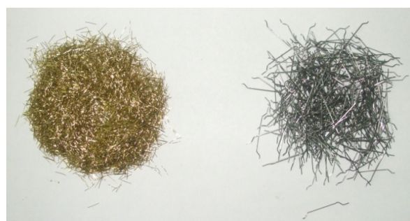
Fig. 5. Long (left) and short (right) steel-fiber reinforcement
