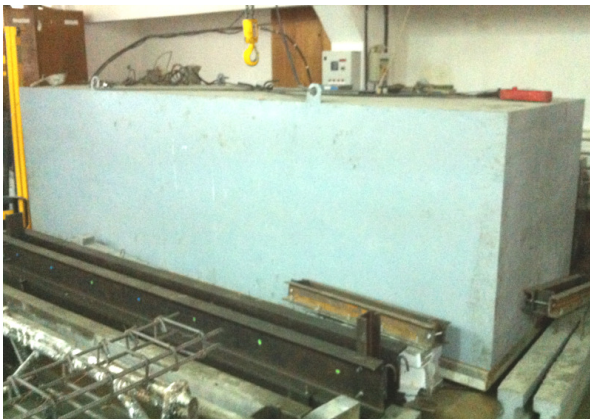
Fig. 3. The oven for applying the thermal treatment
