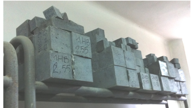
Fig. 4. UHPC samples kept in the climate chamber
