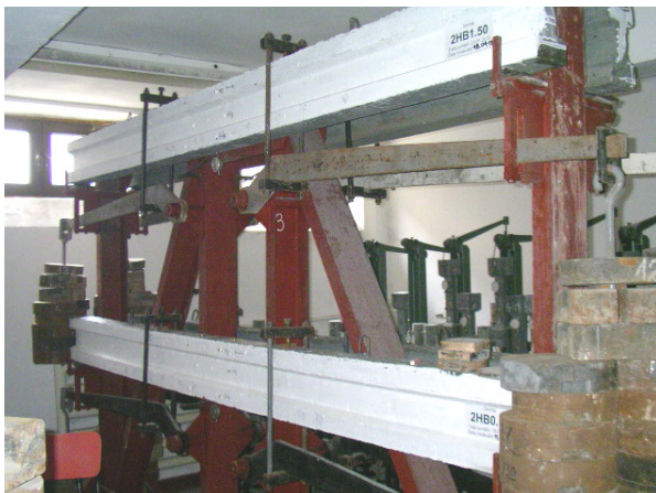
Fig. 7. UHPC beams subjected to long-term bending
