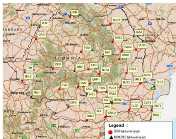
Fig. 8. The distribution of seismic stations in RNS of NIRD URBAN INCERC on the territory of Romania (Dragomir et al. , 2015)
